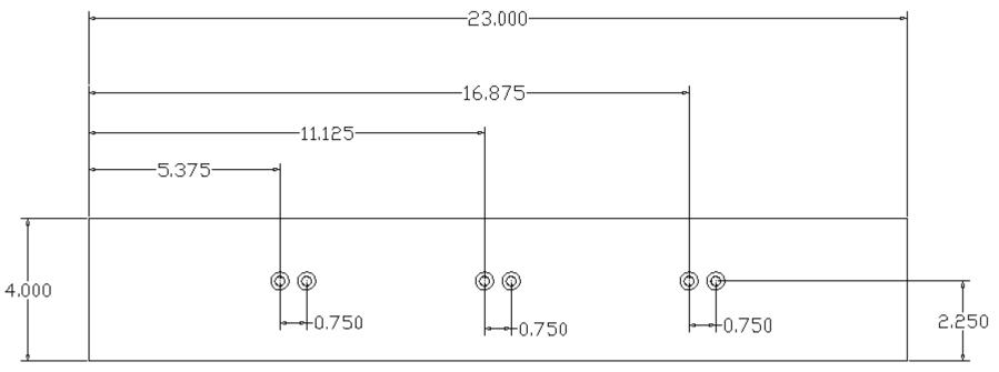
A simple sacrificial fence can be made with any piece of wood. In this example we use a piece of 3/4" MDF cut to 23" x 4". Holes are positioned as shown above, and are 17/64" in diameter with a 1/2" counter bore so the heads of the included screws can sit below the plane of the fence.
